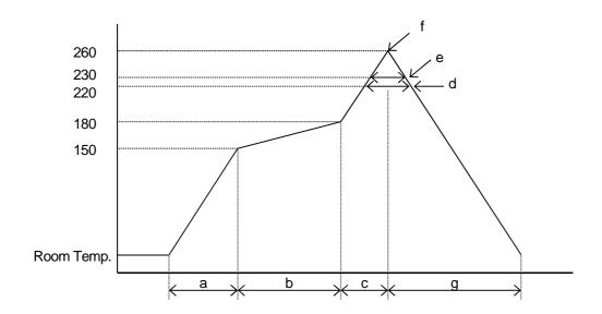
a:Temperature ramping rate :1 to 4 /s : 150 to 180 b: Pre-heating temperature time : 60 to 120s c:Temperature ramp rate :1 to 4 /s d:220 or higher time : Shorter than 60s : Shorter than 40s e:230 or higher time : Lower than 260 f:Peak temperature g:Temperature ramping rate :1 to 6 /s
