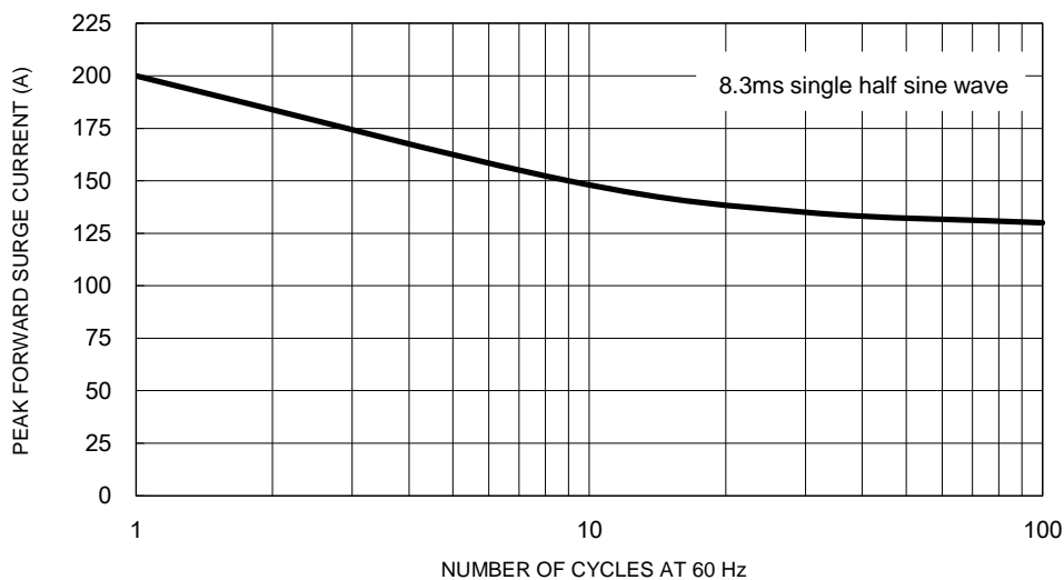
Fig.5 Maximum Non-Repetitive Forward Surge Current
