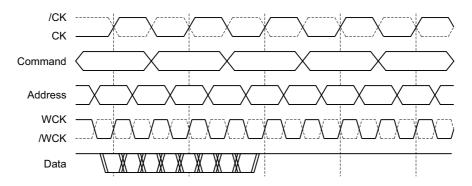
Note: the figure shows the relationship between the data rate of the buses and the clocks and is not a timing diagram.
