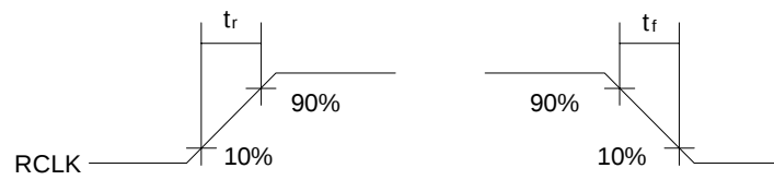
Fig. 12 Signal Rise and Fall Characteristics
