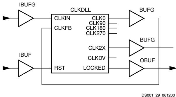
Figure 29: DLL Deskew of Clock and 2x Multiple
