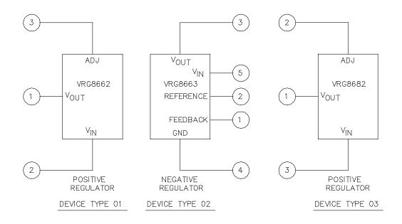
FIGURE 3. Block diagram.
