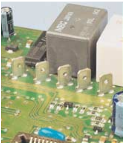
Terminals Inserted with 45° Rotation
