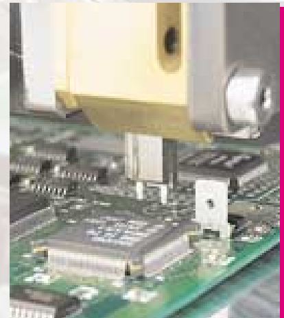
AutoTab Tooling Head Inserting Quick Disconnect Terminal
