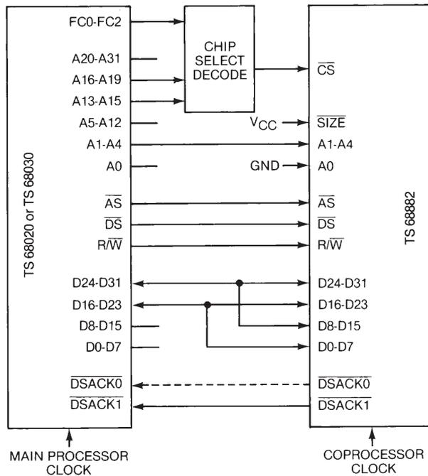
Figure 19 : 16-bit data bus coprocessor connection.
