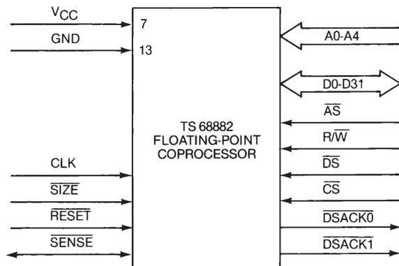
Note : The terms assertion and negation are used extensively. This is done to avoid confusion when describing «active-low» and «active-high» signals. The term assert or assertion is used to indicate that a signal is active or true, independent of whether that level is represented by a high or low voltage. The term negate or negation is used to indicate that a signal is inactive or false.
