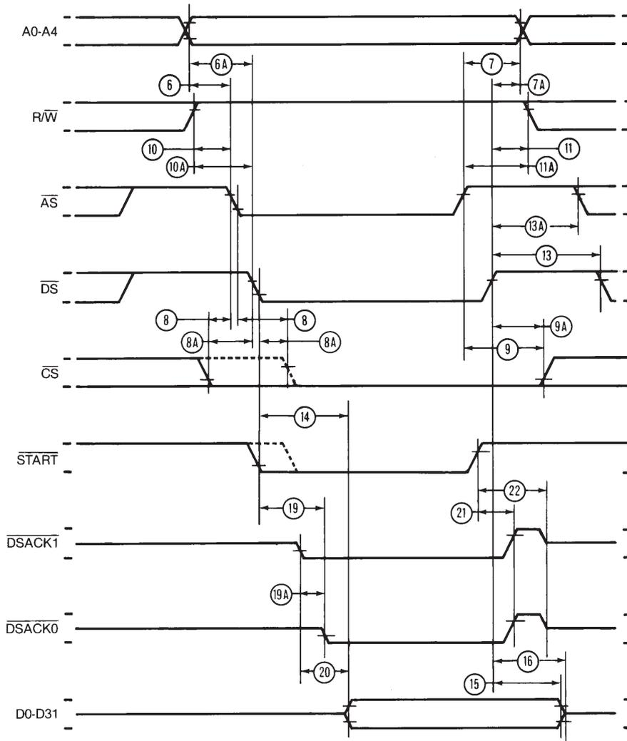
**Note :**  $\overline{START}$  is actually a logical condition, but is shown as an active signal for clarity. The logical equation for this signal is :
