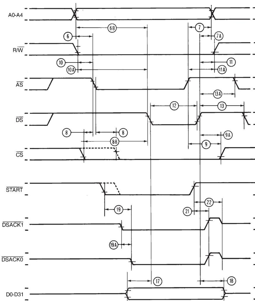
**Note :**  $\overline{\text{START}}$  is actually a logical condition, but is shown as an active signal for clarity. The logical equation for this signal is :
