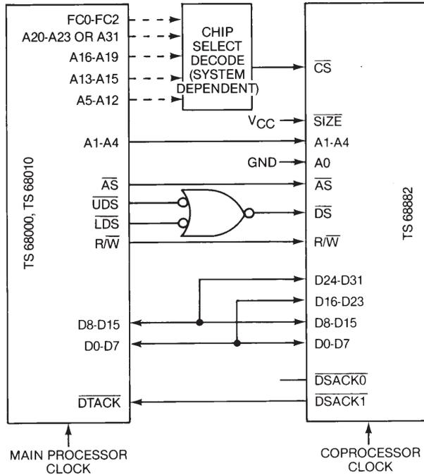
Figure 21 : 16-bit data bus peripheral processor connection.
