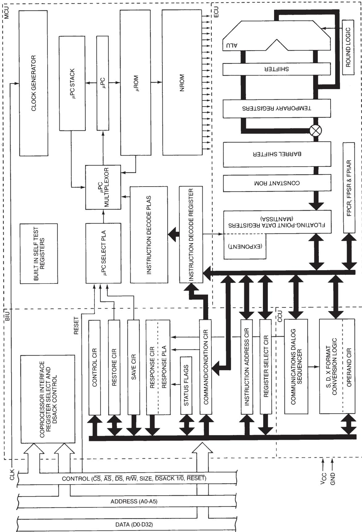
Figure 1 : TS 68882 simplified block diagram.
