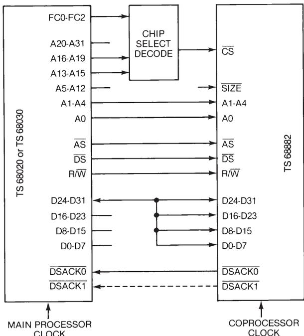
Figure 20 : 8-bit data bus coprocessor connection.
