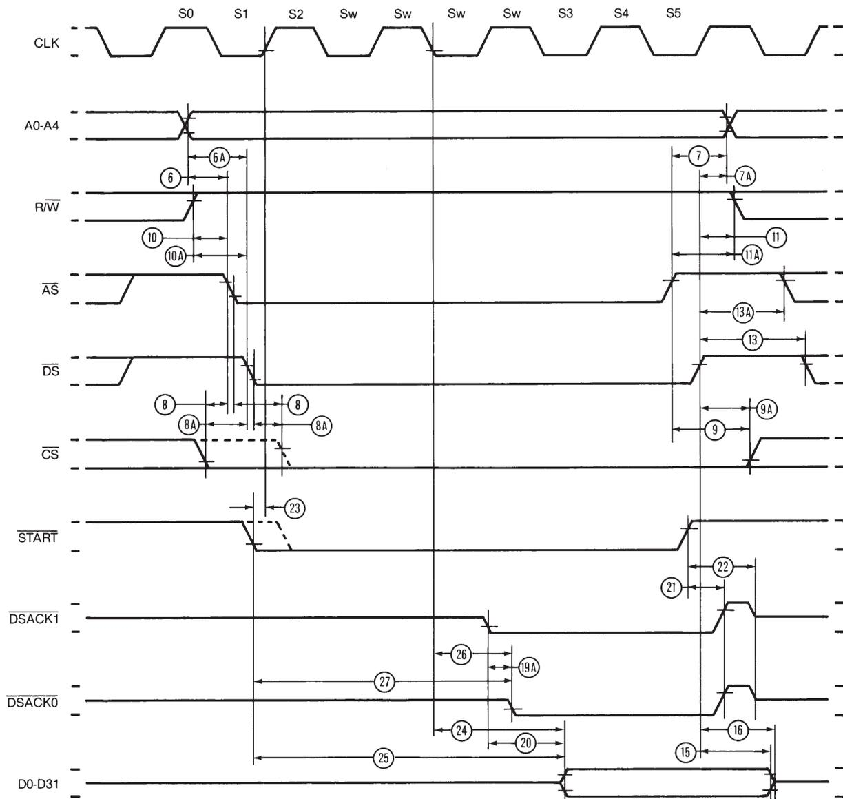
**Note :**  $\overline{\text{START}}$  is actually a logical condition, but is shown as an active signal for clarity. The logical equation for this signal is :
