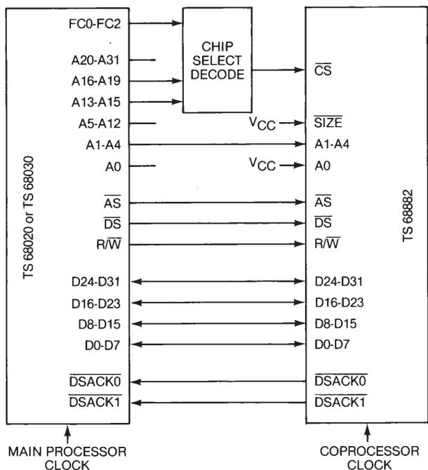
Figure 18 : 32-bit data bus coprocessor connection.
