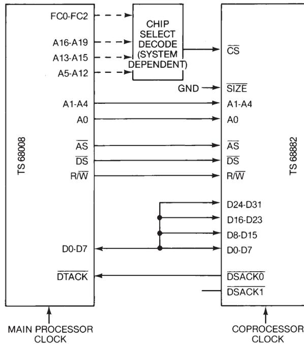
Figure 22 : 8-bit data bus peripheral processor connection.
