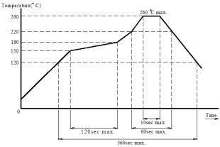
Reflow soldering: Two times max
