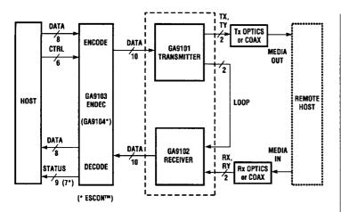
TriQuint's GA9101 Transmitter and GA9102 Receiver, in conjunction with either the GA9103 ENDEC or the GA9104 ENDEC, provide a comprehensive electrical and physical interface in compliance with the Fiber Channel Specification of the Accredited Standards Committee (ASCX3T9.3) or the Enterprise Systems Connection Architecture (ESCON™). These chip sets can also be used for ATM local area network applications operating at serial data rates of 194.4 Megabaud (payload at 155.52 Megabits/sec).
