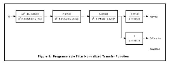
With a zero at the origin, the filter provides a time-differentiated filter output. This is used in time qualification of the peak detection. To ease the timing requirement in peak detection of a signal slightly above the qualification threshold, the time-differentiated output is purposely delayed by 1.2 ns relative to the normal low pass output.
