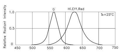
wavelength  $\times$  (nm) RELATIVE INTENSITY Vs. WAVELENGTH
