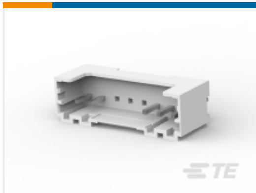
TE Model / Part #1971200-1 GIC 2.0 EV 5/8P HEADER ASSEMBLY
