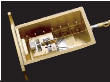
Laser-welded fiber alignment assembly for long-term power stability.
