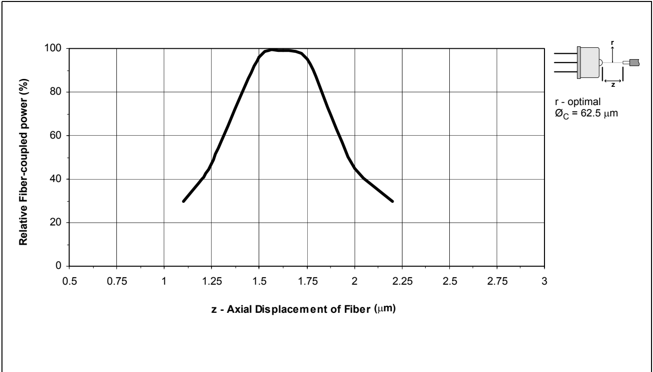
Figure 3 - Relative Fiber-coupled Power vs. z - Axial Displacement of Fiber
