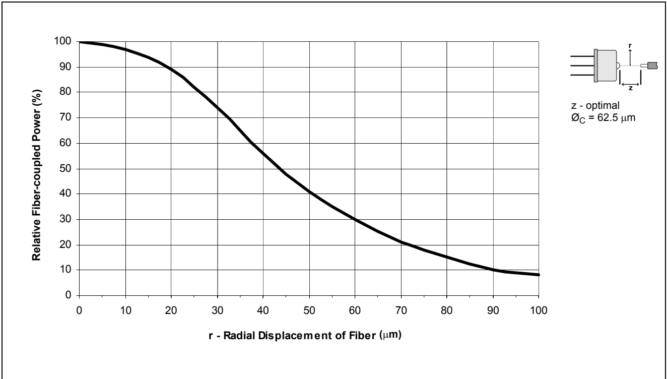
Figure 4 - Relative Fiber-coupled Power vs. r - Radial Displacement of Fiber
