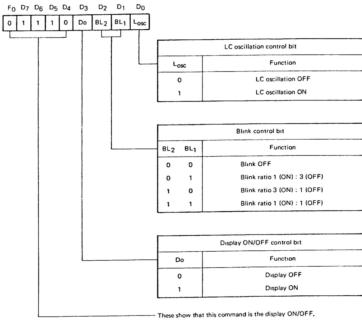
These show that this command is the display ON/OFF, blink and LC oscillation command.
