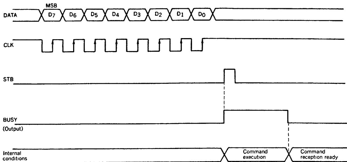
For format data, a busy signal is generated after the internal conditions are completely determined. When writing data in VRAM, a busy signal is generated after the completion of writing in VRAM. When the VRAM write period extends into the horizontal retrace line period, the busy signal becomes longer than usual, so be careful. (This is because oscillation is suspended during the horizontal retrace line period, so writing in VRAM becomes impossible.)
