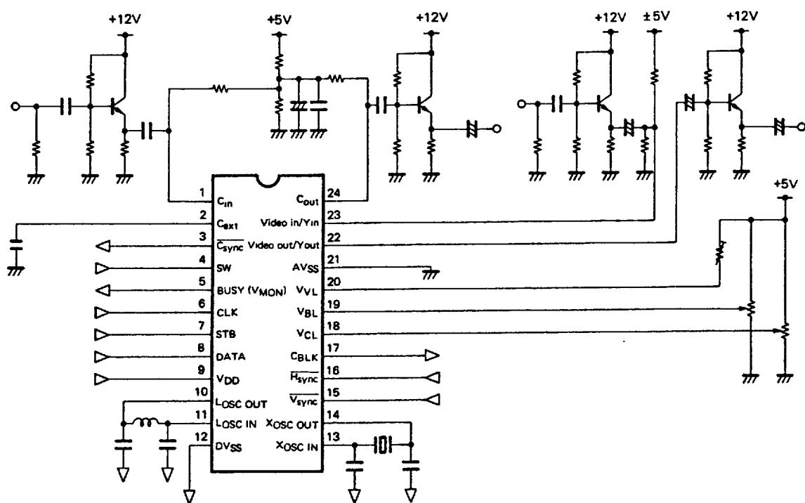
Note: The peripheral amplifier uses +12 V. To use +5 V, give attention to the amplifier configuration.
