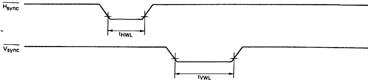
RECOMMENDED OPERATION TIMING ( $T_a = 25^\circ\text{C}$ ,  $V_{DD} - V_{SS} = 5.0\text{ V}$ )
