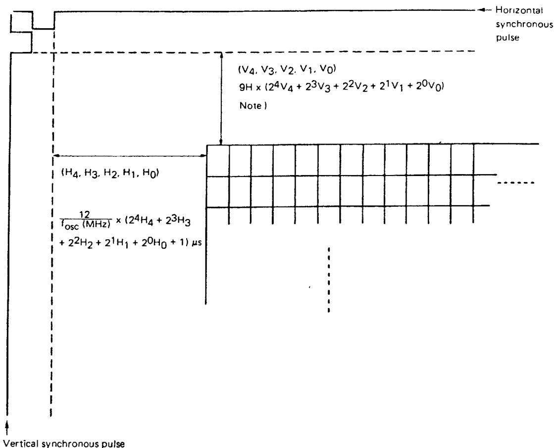
**Note:** Vertical address counter is incremented by the leading edge of the horizontal synchronous pulse.
