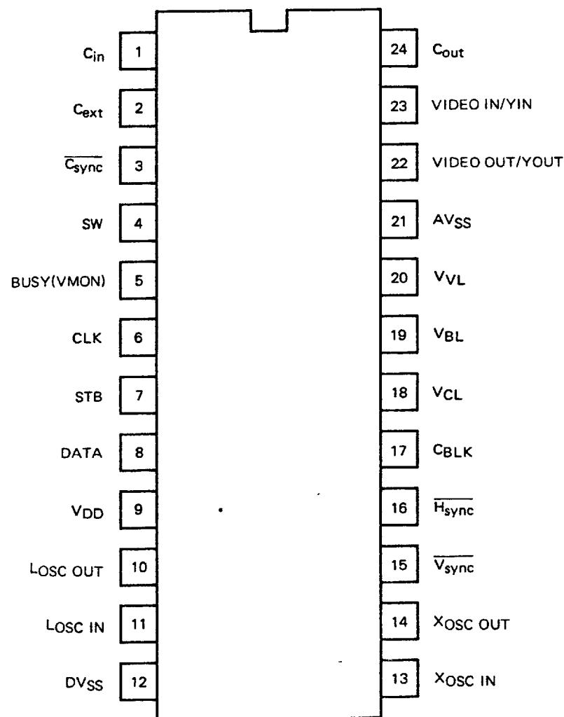
Note: This bracket shows terminal arrangement for the mask code option when terminal 5 of μPD6452 is used for the synchronization protection monitor output (VMON)
