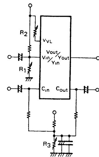
Note: Since there is no built-in pedestal clamp circuit for external video signal, connect direct current clamp circuit in front of "video in/Y in".
