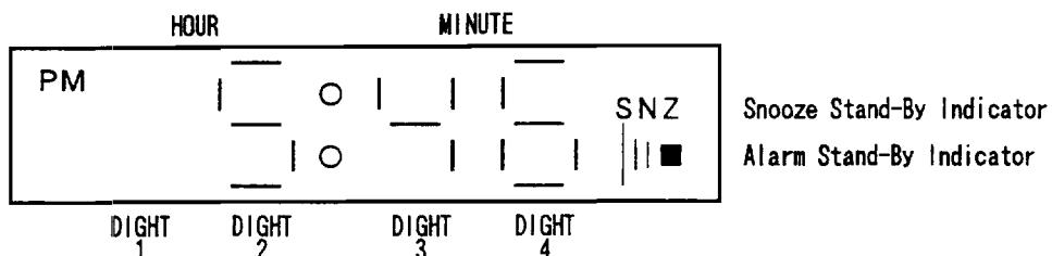
In this mode, the current time is displayed. If the time is afternoon, the "PM" indicator is also ON. If the HOUR is less than 10, the DIGIT 1 is not displayed.
