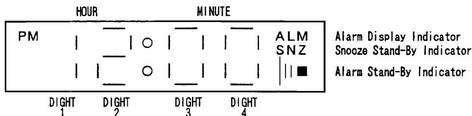
In this mode, the alarm time is displayed. If the time is afternoon, the "PM" indicator is also ON. If the HOUR is less than 10, the DIGIT 1 is not displayed.
