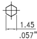
Recommended Crimped Dimensions for Center Pin
