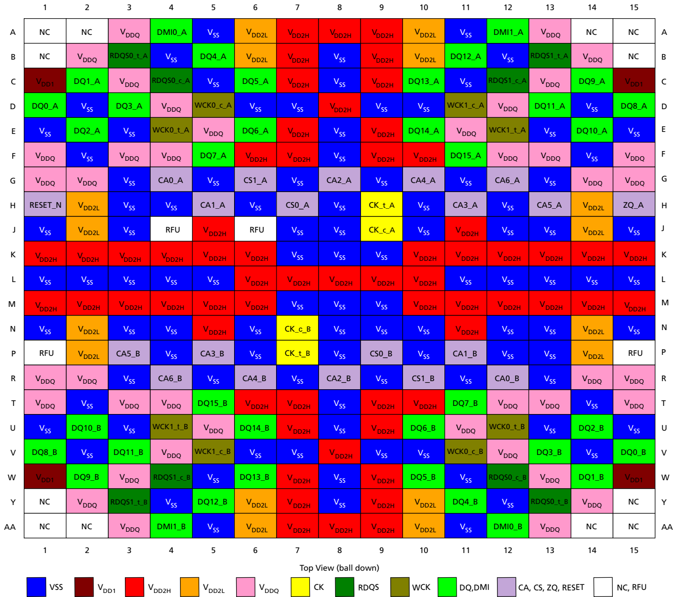
Figure 4: 315-Ball Dual-Channel Discrete FBGA
