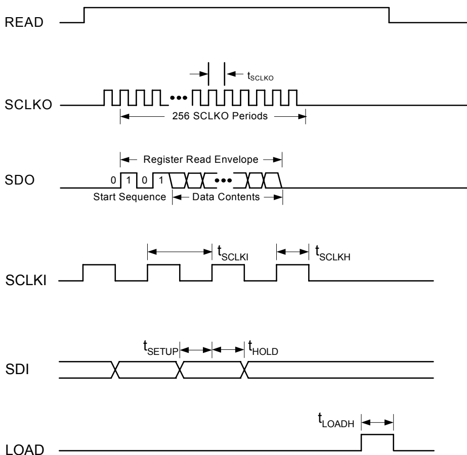
Figure 5. Output Phase Adjust Timing Diagrams (Register Control)
