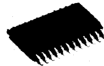
Outline 24P2W-A 1.27mm pitch 450mil SOP (8.4mm×15.0mm×2.0mm)
