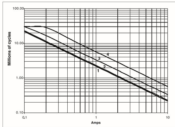
DC Current breaking capacity  $L/R = 20 \text{ ms} ; 40 \text{ ms}$
