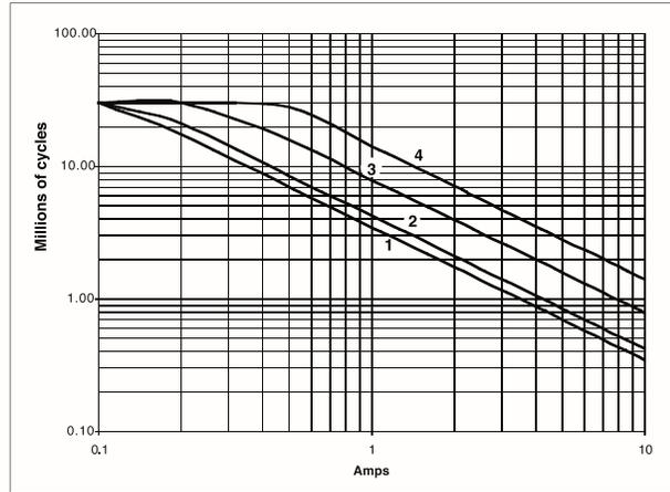
AC Current breaking capacity at  $\cos\phi = 0.7 ; 0.5 ; 0.3$
