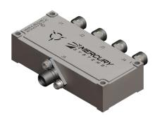
The Mercury Syetms PIN diode SP4T switch family spans the frequency range of 0.5 – 18 GHz. It offers high performance and an integrated high speed driver controlled by TTL or CMOS signals. This switch will maintain high performance as a drop in device for system or subsystem requirements. The Mercury Systems family of high performance switches is available in military or non military versions, hermetic and non-hermetic.
