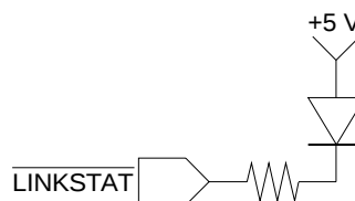
Figure 6. LED Connection Diagram
