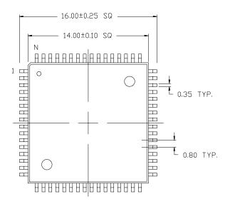
DIMENSIONS IN MILLIMETERS LEAD COPLANARITY 0.102 MAX.
