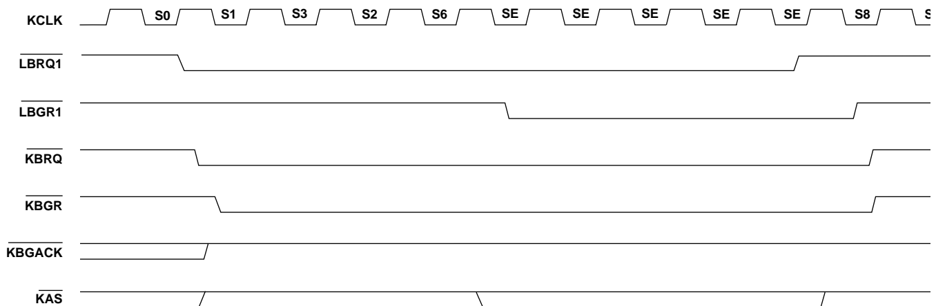
Figure 2.19 : Local Arbitration for External Device - Without Acknowledgment
