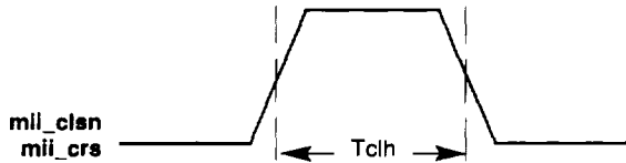
Figure 14 MII/SYM Port Timing Diagram—Carrier Sense and Collision
