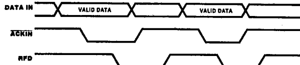
Figure 21. Interlocked Handshake Timing (Input) Port 2 Side Only
