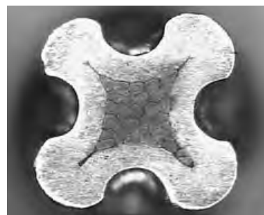
Cross-section 8-point crimping
