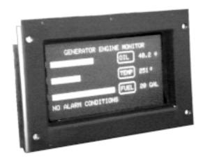
The APD-192G088-5 is a full field dot matrix display with 192 columns and 88 rows. It includes drive electronics, microprocessor based controller, IR touch panel and bezel. The controller maintains all the refresh memory, character generation, touch input and control logic to enable the module to serve as a direct input/output device for communications terminals, computer readouts, microprocessor instruments or any other system requiring a self-contained input/output terminal.
