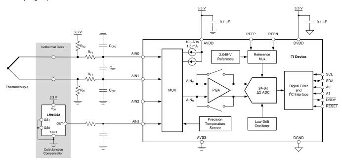
Figure 71. Thermocouple Measurement
