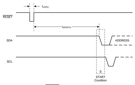
Figure 2. RESET Pin Timing Requirements
