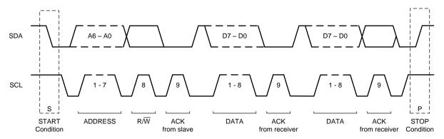
Figure 55. I<sup>2</sup>C Data Transfer Format
