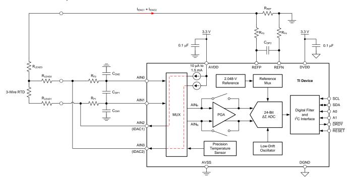
Figure 74. 3-Wire RTD Measurement
