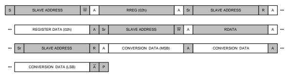
Figure 61. Using the DRDY Bit to Check for New Conversion Data
