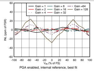
Figure 13. INL vs Differential Input Voltage
