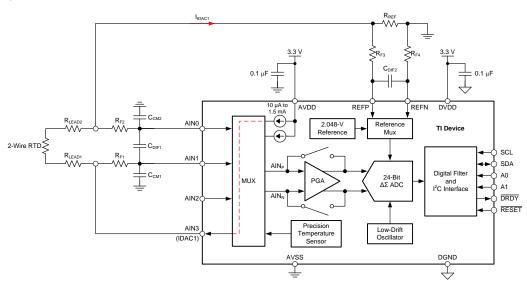
Figure 75. 2-Wire RTD Measurement
