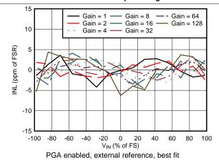
Figure 12. INL vs Differential Input Voltage
