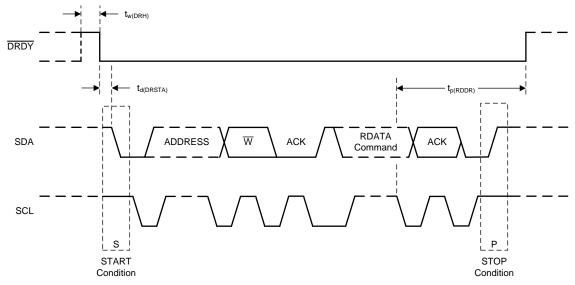
Figure 3. DRDY Pin Timing Requirements and Switching Characteristics
