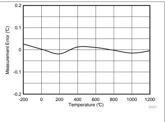
Figure 73. Temperature Measurement Error vs T<sub>(TC)</sub>
