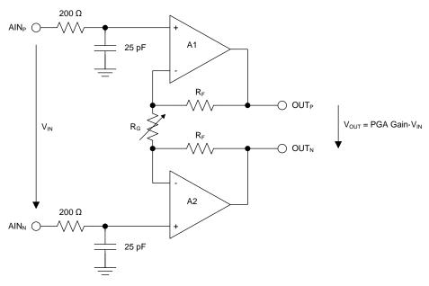
Figure 43. Simplified PGA Diagram
