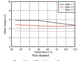
Figure 15. Input Offset Voltage vs Temperature
