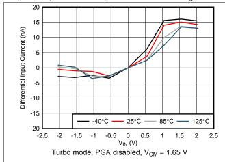
Figure 10. Differential Input Current vs Differential Input Voltage
