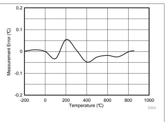
rror vs R<sub>RTD</sub> Figure 78. Temperature Measurement Error vs T<sub>(RTD)</sub>
