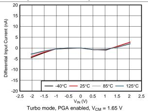
Figure 11. Differential Input Current vs Differential Input Voltage
