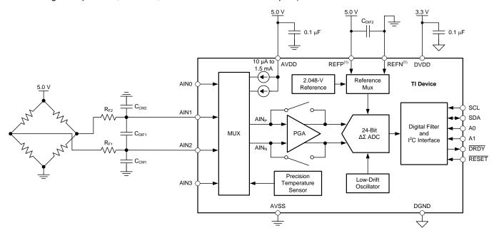
(1) Connect reference inputs directly to the bridge excitation voltage through Kelvin connections.
