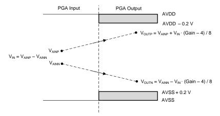
Figure 44. PGA Input/Output Voltage Relationship
