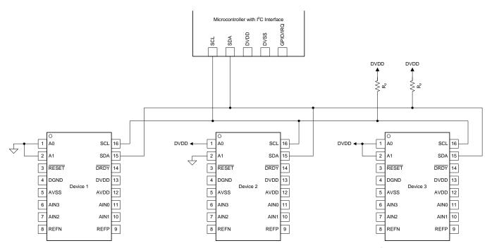
Figure 69. Connecting Multiple ADS122C04 Devices on the Same I<sup>2</sup>C Bus
