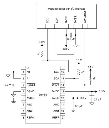
Figure 68. Interface Connections
