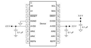
Figure 80. Unipolar Analog Power Supply
