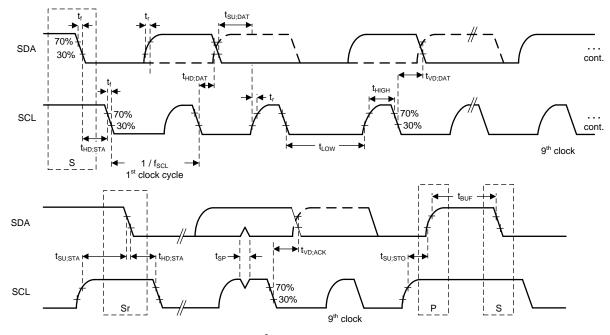
Figure 1. I<sup>2</sup>C Timing Requirements
