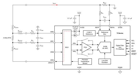
Figure 76. 4-Wire RTD Measurement
