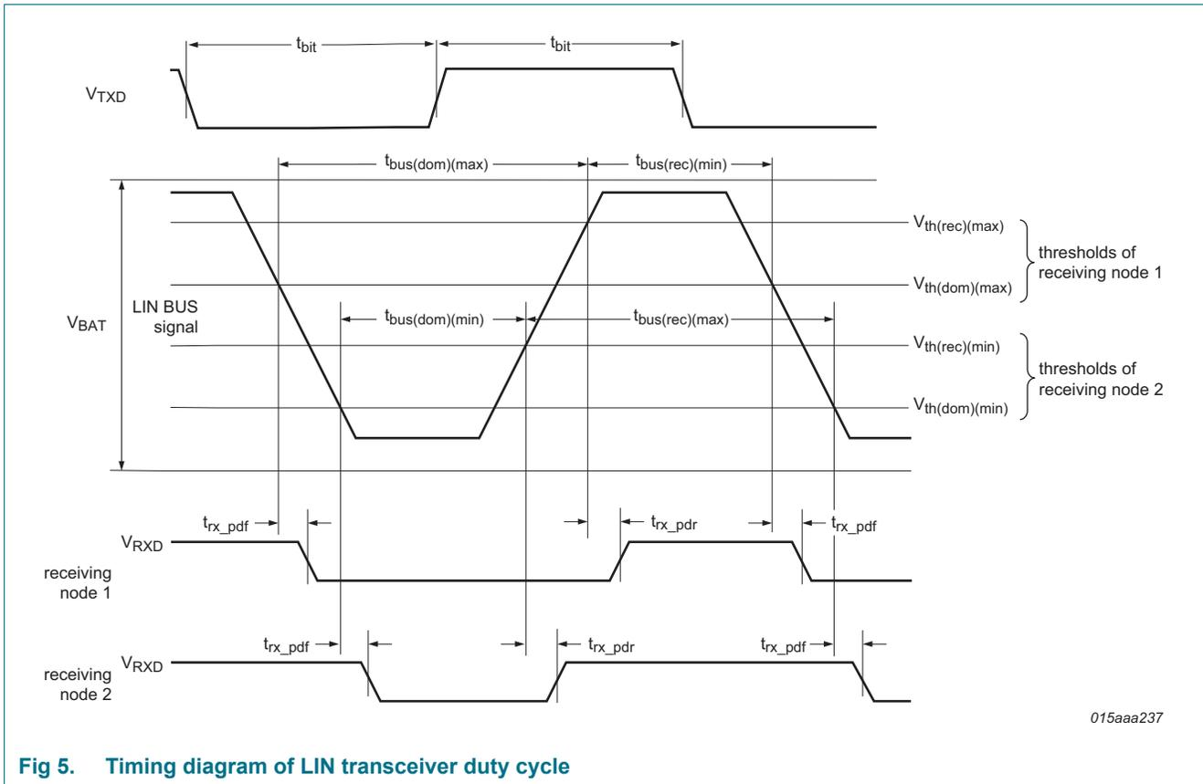
**Fig 5. Timing diagram of LIN transceiver duty cycle**
