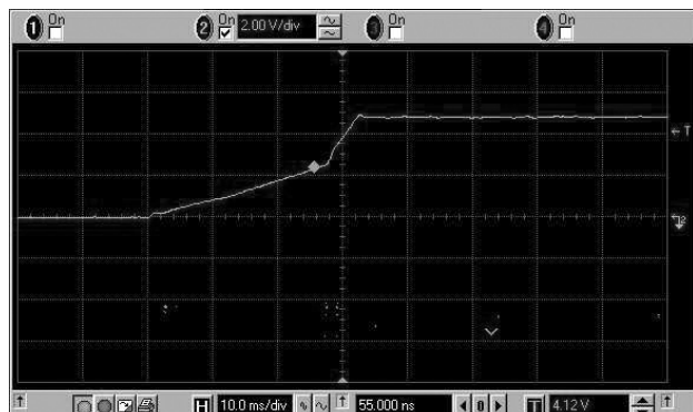
Rise Time (PWM mode): V_{in} = 4.5V ; V_{TP} = 5V ; I_{out} = 2A
