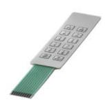
Membrane keypad, self-adhesive, silver conduction technology, 12 keys, embossed, 3 colors, connection cable: 88.5 mm, with crimp female connector RM 2.54 mm, operating temperature -20 °C ... 70 °C
