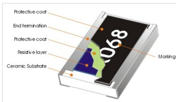
Fig 2. Construction of a 1218 Chip-R
