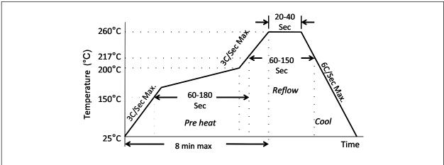
FIGURE 7-1: Solder Reflow Profile.
