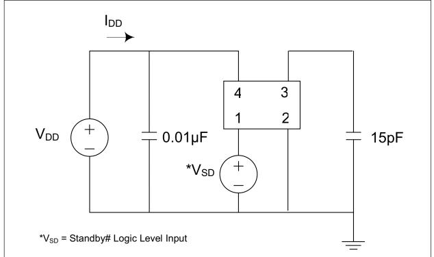
FIGURE 5-1: DSC1001/3/4 Test Circuit.
