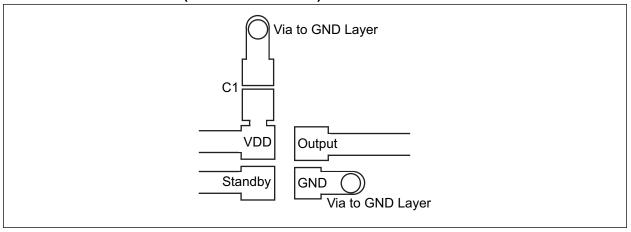
FIGURE 6-1: Recommended Board Layout for DSC1001/3/4.
