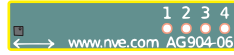
AG904-06: DFN4 connection board for -14E suffix sensors. (1.2" x 0.25" / 30 mm x 6 mm; actual size).
