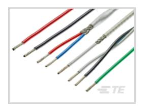
Cable Type: Spec 44 Voltage Rating: 600 VAC Insulation Material: Modified Radiation Cross-linked PVDF Conductor Material: Tin-Coated Copper Wire Size: 26 AWG
