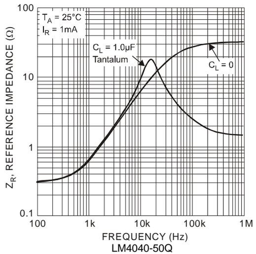
**Typical Characteristics – LM4040Q Noise Characteristics**
