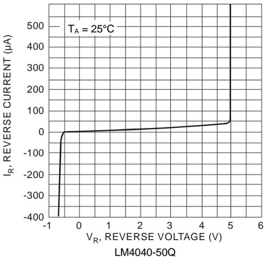
**Typical Characteristics – LM4040Q Reference Impedance**
