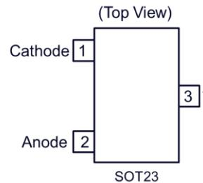
\* Pin 3 must be left floating or connected to pin 2
