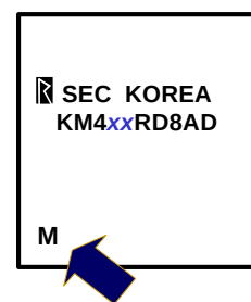
b. Top marking example of mirrored package
