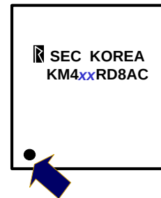
b. Top marking example of normal package
