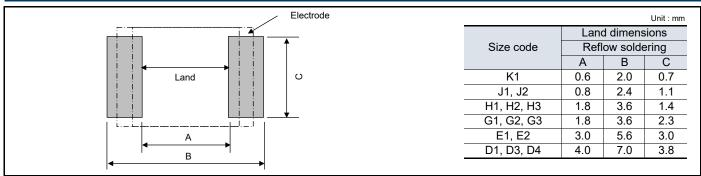
\* It is not warrantable that you can mount the capacitor without trouble under all the mounting condition when "Recommender for Land dimensions" is adopted.
