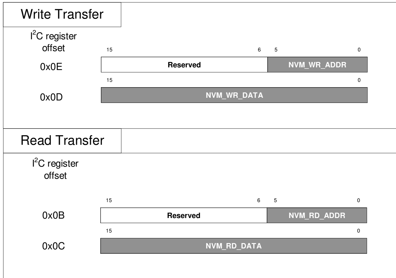
Figure 9-12. EEPROM Direct Access Using I 2 C
