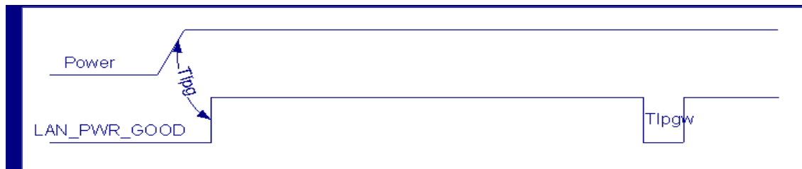
Figure 12-7. External Reset Timing Diagram
