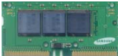
Figure 1: SO-RIMM Module shown with heat spreader removed
