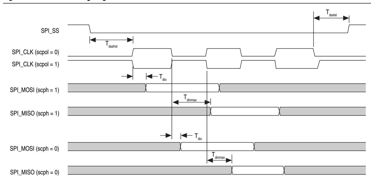
Table 39 lists the SPI slave timing characteristics for Cyclone V devices. The setup and hold times can be used for Texas Instruments SSP mode and National Semiconductor Microwire mode.
