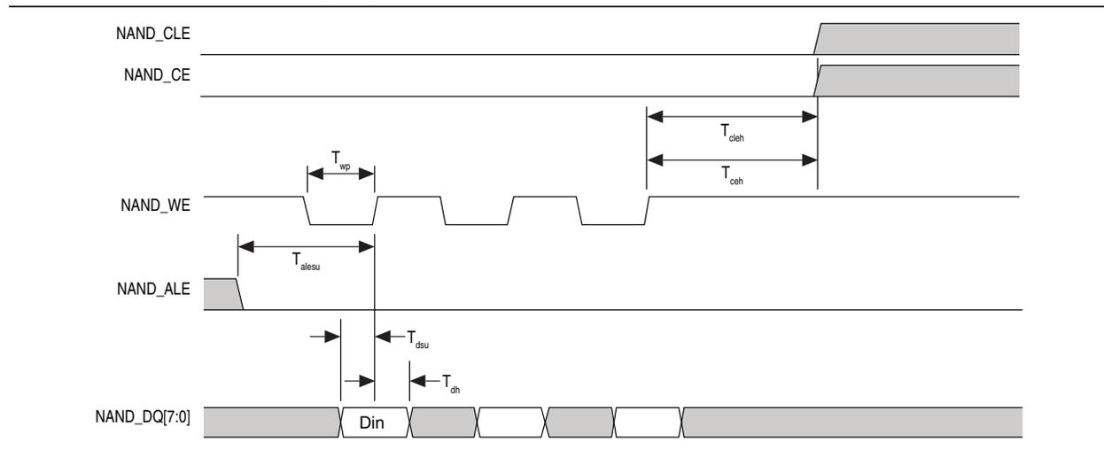
Figure 16 shows the timing diagram for NAND data read timing characteristics.
