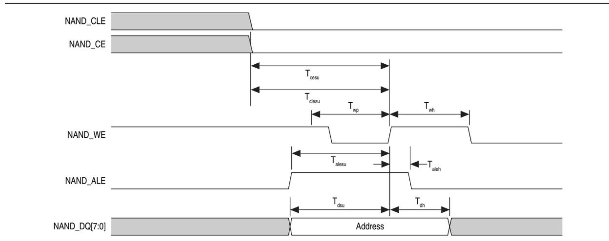
Figure 15 shows the timing diagram for NAND data write timing characteristics.
