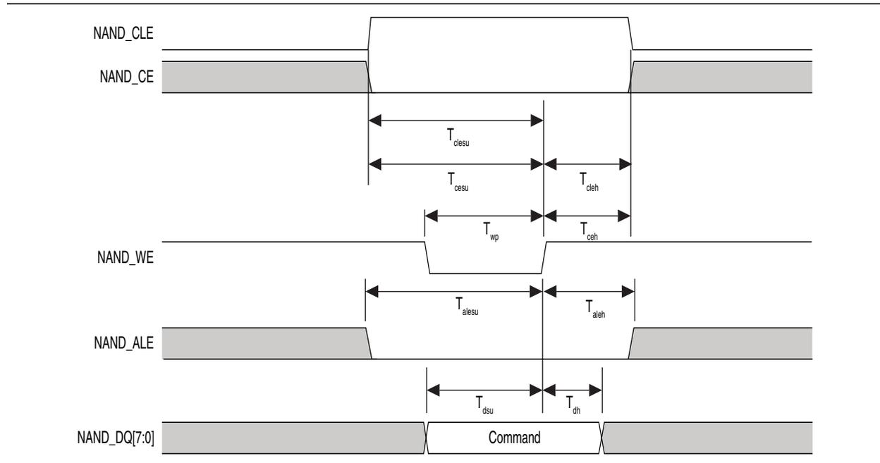
Figure 14 shows the timing diagram for NAND address latch timing characteristics.
