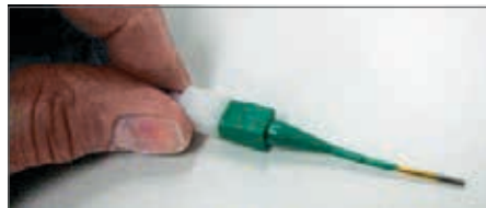
Plastic tool with contact in proper position.
