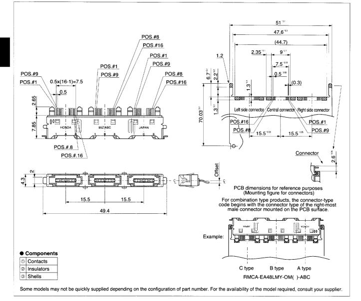
Mating connectors: RMCA series of soldering type female connectors
