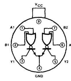
Pin 4 is in electrical contact with the case.
