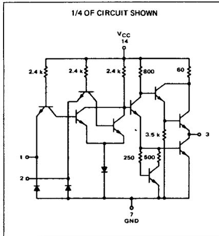
This device consists of four 2-input OR gates. This non-inverting function is useful for optimizing logic design, or for direct implementation of standard logic equations.
