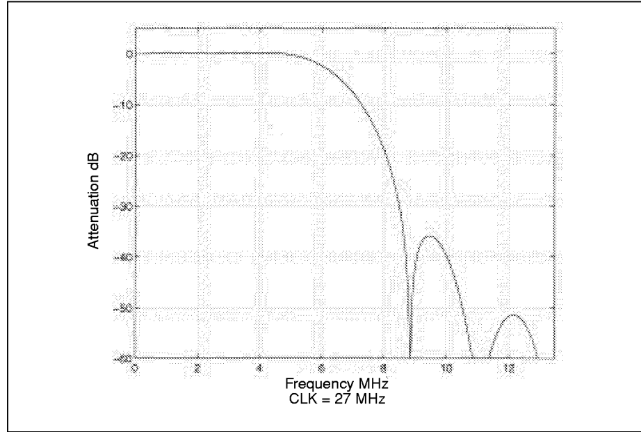
Figure 11a. Luminance 2X Upsampling Filter Response
